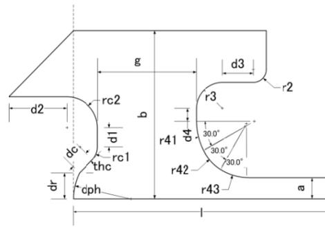
Figure 2: First cavity shape and searched parameters
