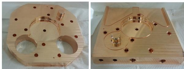
Figure 8: Photo of manufactured cavity cell
