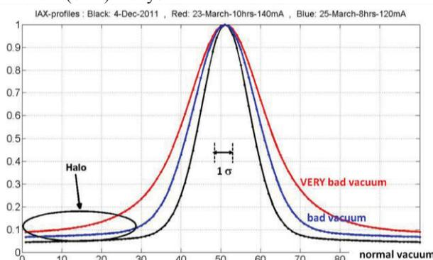
Figure 1: X-ray projected profiles at different vacuum conditions before and after shut-down (red and blue).
