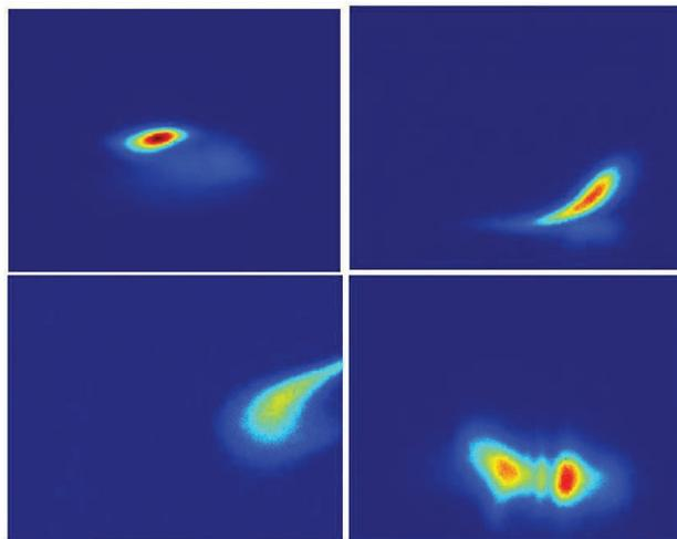
Figure 4: Images of the transverse beamsize of the injected beam at the first 4 turns in the Ring. The hor. and vert. scales are respectively ~16 and ~12mm.
