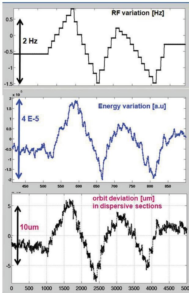
Figure 3: An 8 minutes recording of the RF frequency variation [Hz], the relative energy fluctuation, and the horizontal orbit deviation (in dispersive sections) [um].
