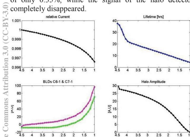
Figure 2: Recordings of relative beam current, Lifetime, BLDs and the amplitude of the Halo detector during a rapid scan of the scraper from 4.5 to 1mm.
