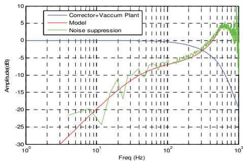
Figure 8: Simulation of noise sensitivity function of the FOFB system.
