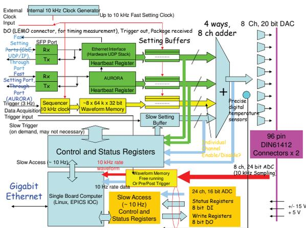
Figure 4: Functional block diagram of the corrector power supply controller module. Fast setting from orbit feedback and slow setting from EPICS CA console.
