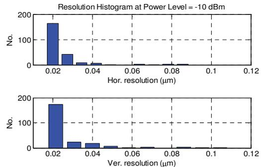
Figure 1: Histogram of horizontal and vertical position resolution distribution at power level around -10 dBm for 228 BPM modules.
