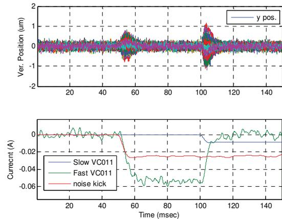
Figure 9: Transaction simulation when the fast corrector DC setting is transfer red to the nearby slow corrector.
