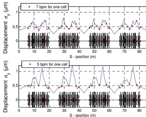
Figure 7: Static simulation for FOFB shown in 4 cells.
