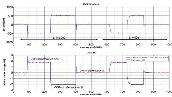
Figure 3: FOFB GDX closed loop test. The upper plot is position; the lower plot is relative power level change.
