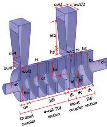
Figure 8: 3D model of the Hybrid Buncher.
