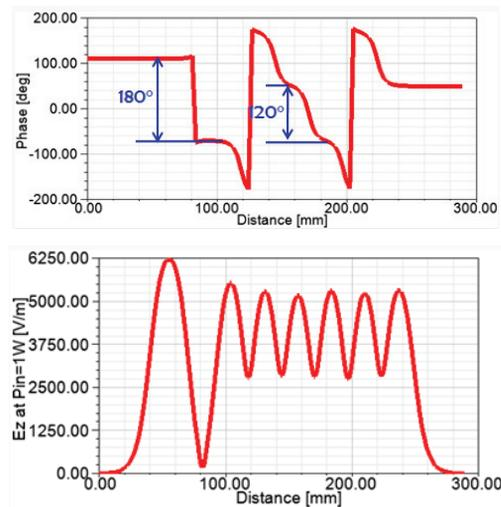
Figure 10: Phase (upper) and amplitude (lower) distribution along the axis of the Hybrid Buncher.
