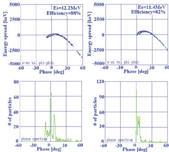
Figure 4: Spectrums at the bunching system exit (left for nominal bunching system; right for HB bunching system).
