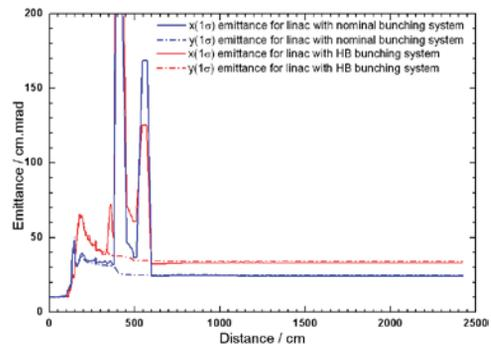
Figure 7: Emittance evolution along the linac.
