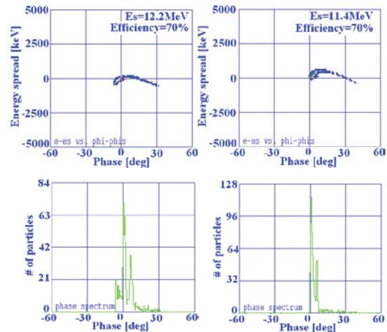
Figure 5: Spectrums at the chicane system exit (left for nominal bunching system; right for HB bunching system).
