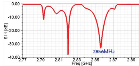
Figure 9: S11 at the RF input coupler port.
