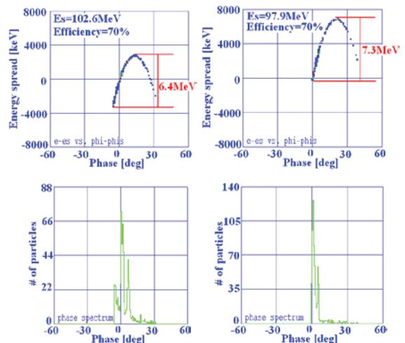
Figure 6: Spectrums at the linac exit (left for nominal bunching system; right for HB bunching system).
