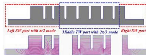
Figure 2: Initial 2D design of the HB by SUPERFISH.
