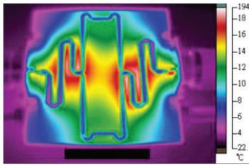
Figure 7: The back-to-back connection of Y-junction power divider/combiner for insertion loss and temperature distribution measurement.
