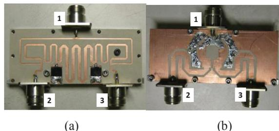
Figure 3: The designed 500MHz two-way (a) Gysel and (b) balance power divider/combiner.
