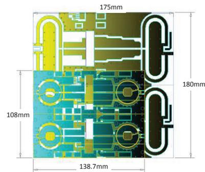
Figure 1: Dual SSPA using coaxial and planar balun in parallel for size comparison.
