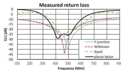
Figure 4: The input return loss of the four fabricated power dividers/combiners.
