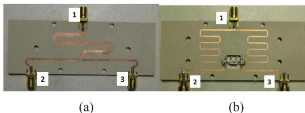
Figure 2: The designed 500MHz two-way (a) Y-junction and (b) Wilkinson power divider/combiner.
