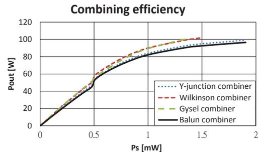
Figure 9: The combining efficiency of the four dividing/combiner methods.
