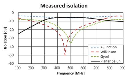
Figure 5: The measured isolation between port 2 and 3 of the four power dividers/combiners.
