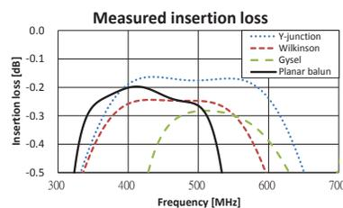
Figure 6: The insertion loss investigation by back-to-back connection of the four methods as in Fig. 9.
