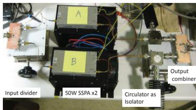
Figure 8: The setup for power combining efficiency using two identical 50W SSPAs.
