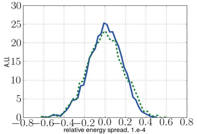
Figure 3: Energy spread  $\gamma/\gamma_0$  at the undulator exit, from initially delta-distributed beam. Direct Monte Carlo (solid) and stochastic integration (dashed), for 17.0 GeV Beam, K=1.0, over 100m
