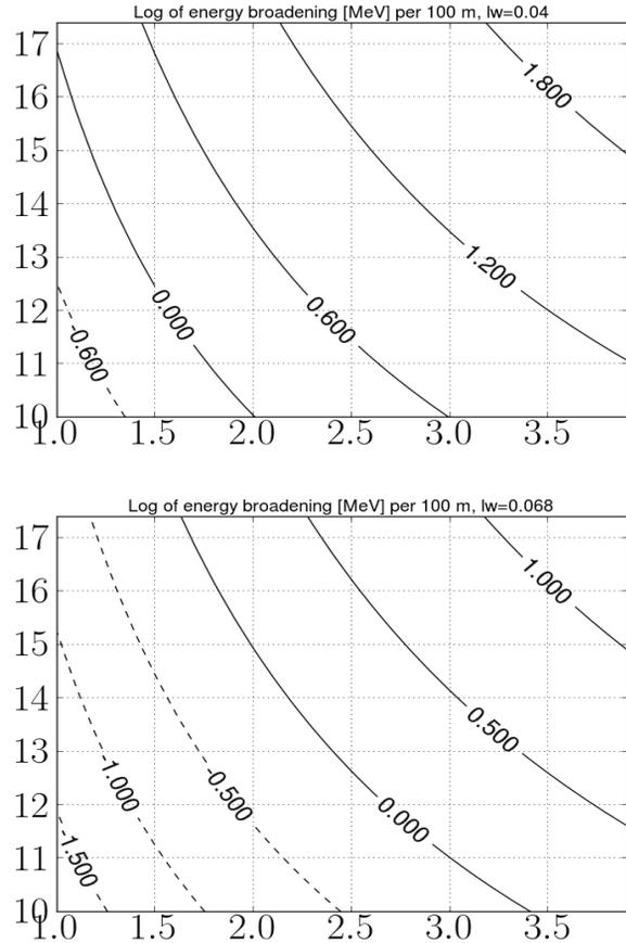
Figure 1: Diffusion coefficients for SASE XFEL undulators. Vertical axis is beam energy, horizontal is  $K$
