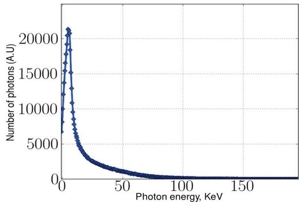
Figure 4: Spectrum of emitted photons E=17.0 GeV, K=1.0
