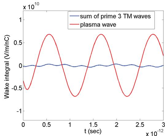
Figure 3: Time profile of the longitudinal wakefields of the prime 3 TM waves (blue) and the plasma wave (red).
