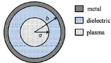
Figure 1: Cross-section of a plasma filled dielectric tube.
