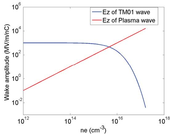
Figure 4: Wake amplitude of the  $\text{TM}_{01}$  wave (blue) and the plasma wave (red) as functions of plasma density.
