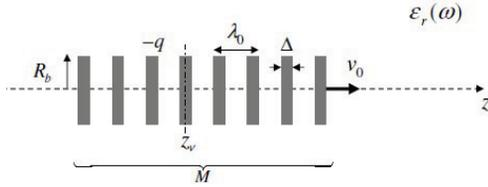
Figure 3: A macro-bunch consisting of a train of  $M$  micro-bunches traversing a medium characterized by its dielectric coefficient  $\epsilon_r(\omega)$ . Each micro-bunch carries a charge  $-q$ .
