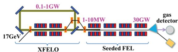
Figure 3: XFELO seeded high-gain FEL configuration.
