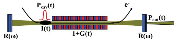
Figure 1: Schematic and brief model of an XFEL.
