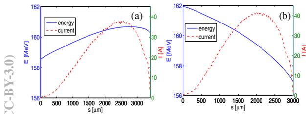
Figure 2: Beam energy and current distributions (bunch head is to the right) at the exit of the linac for two cases: (a) normal electron beam; (b) chirped electron beam.
