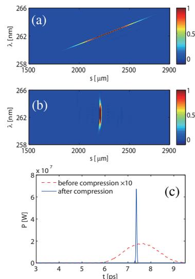
Figure 4: Wigner distributions of the output radiation pulses before (a) and after (b) the optical compressor, and the comparison of output radiation pulses.
