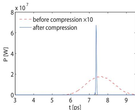
Figure 5: A comparison of the output radiation pulses before and after compressor.
