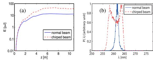
Figure 3: FEL performance for normal electron beam and chirped electron beam: (A) Radiation energy as a function of the radiator undulator length; (B) spectra at saturation.
