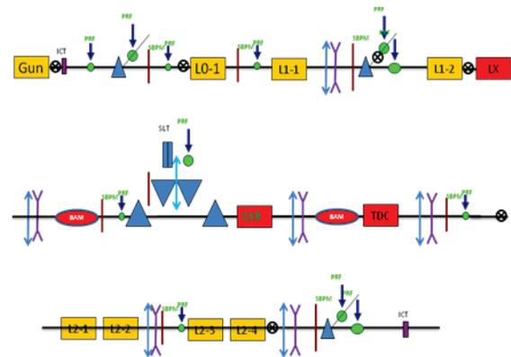
Figure 6: Elements and instruments along the beam line and red coloured blocks are reserved space for future upgrade
