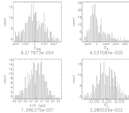
Figure 3: Average beam energy (on the top left), energy spread (on the top right), arrive time (on the down left) and bunch length (on the down right) jittered values obtained by randomly sampling input linac parameters.
