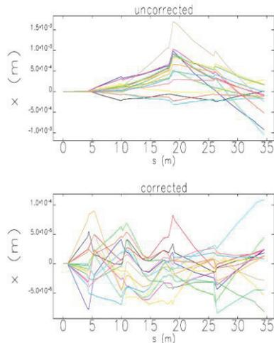
Figure 4: Beam orbit along beamline before (up) and after (down) beam correction techniques are adopted.
