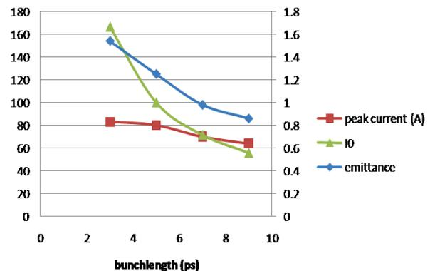
Figure 2: The emittance dilution effect and bunch lengthening process depending on the different initial bunch length.
