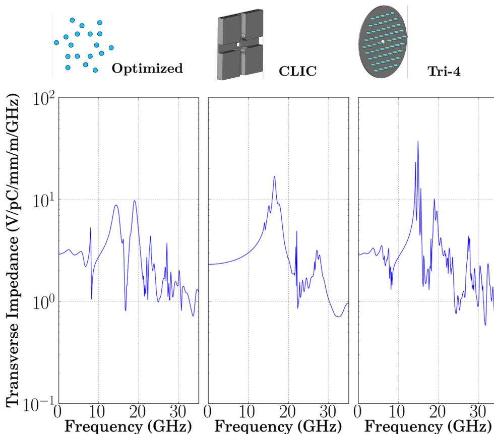
Figure 3: Fourier transform of transverse wake-fields for different structures. The wake-fields for the optimized PhC structure are significantly lower those of the lattice structure.
