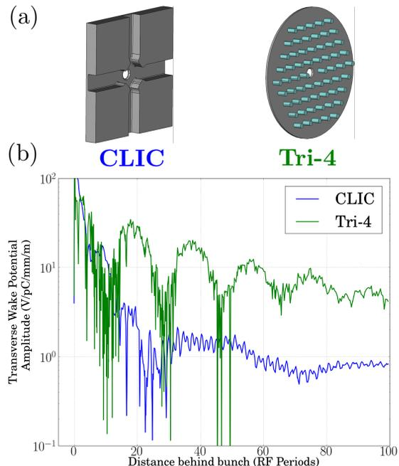
Figure 1: (a) Cross-sections of the CLIC and Tri-4 Cavities. (b) Wake-field comparison of CLIC and Tri-4 cavities. Computational calculations [7] are done for 8-cell 3D cavities.
