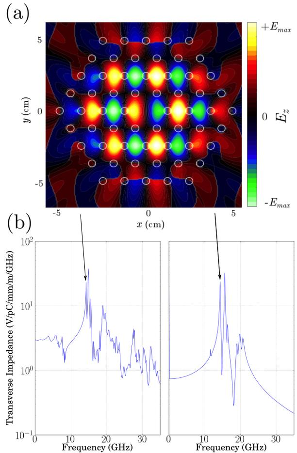
Figure 2: (a) Dipole mode extracted at the frequency shown in the plot below. (b) Fourier transform of transverse wake-fields for the 8-cell 3D cavity (left) and reconstructed wake-fields from the 2D  $k_n$  (right).
