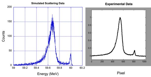
Figure 3: Energy profiles (simulated on the left, experimental on the right) of an electron beam after it has traversed the MAP in the absence of laser fields. The large, lower energy peak corresponds to electrons that have lost energy by scattering with the dielectric materials. The smaller, higher energy peak corresponds to electrons that have passed through the vacuum channel.
