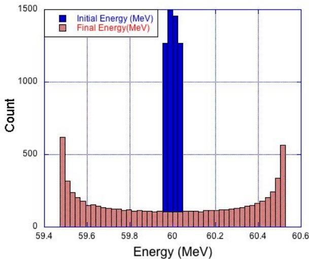
Figure 4: Simulated energy histogram of electron beam after it has passed through the MAP with (red) and without (blue) the accelerating mode excited. Energy modulation due to the accelerating mode results in a broader, double-peaked distribution. Bins are 20 keV wide.
