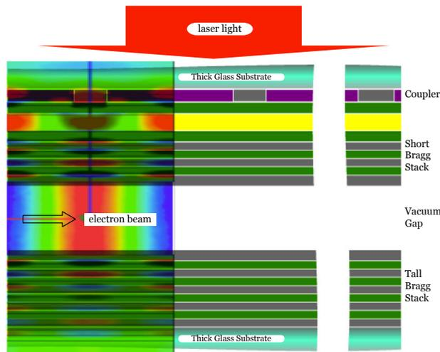
Figure 1: A cross-section of the MAP showing 3 structural periods. An infrared laser pulse is incident upon the structure from above; axial fields of the resulting accelerating mode are shown overlaid on the first structure period (red corresponds to positive values, blue negative). Electrons are accelerated synchronously along the  $\pi$ -mode standing wave resonance.
