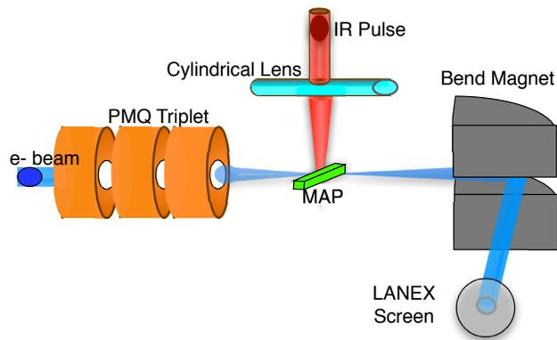
Figure 2: A diagram of the final section of the NLCTA beamline, including the interaction with the MAP. The electron beam is focused to a small spot at the MAP's location, where an IR laser pulse excites the accelerating mode. Downstream of the MAP, the right angle bending magnet is an energy spectrometer.
