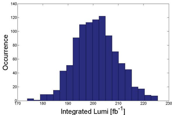
Figure 2: Distribution of integrated luminosity for HL-LHC, based on figures from 2012 operation.
