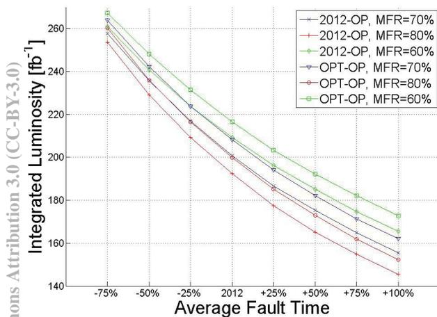
Figure 3: Integrated luminosity versus fault time. Different curves are presented for 2012-like (2012-OP) and Optimized (Opt-OP) operation, for different Machine Failure Rates (MFR).
