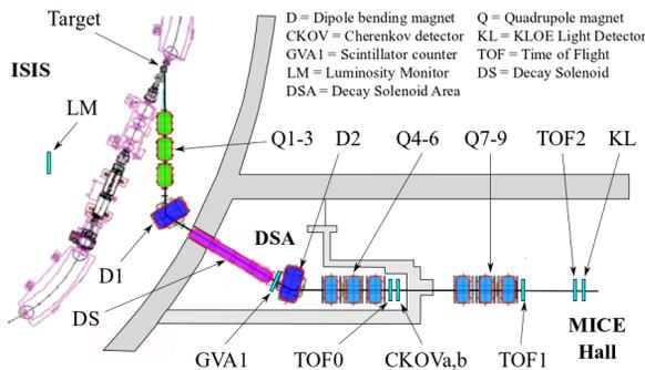
Figure 1: The MICE beamline at step 1.
