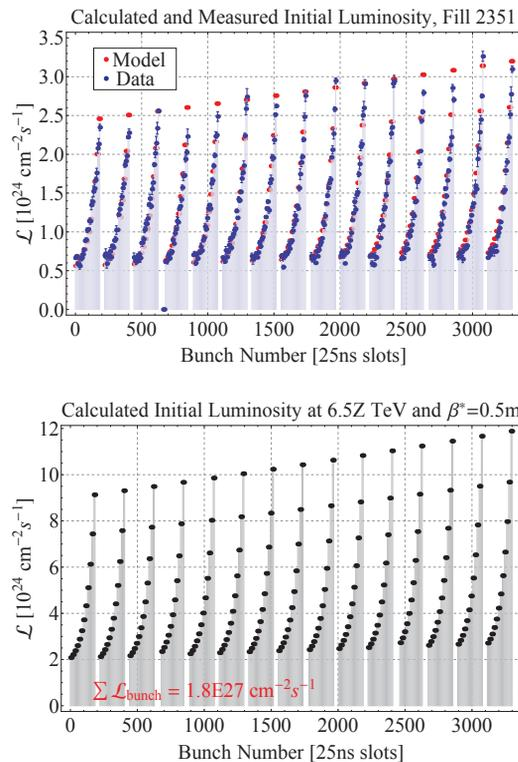
Figure 5: Bunch-by-bunch model ( $E = 3.5Z \text{ TeV}$ , top) and estimate ( $E = 6.5 \text{ TeV}$  bottom) of the initial luminosity.
