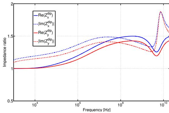
Figure 5: Ratio between the transverse dipolar impedances before and after the scraping.
