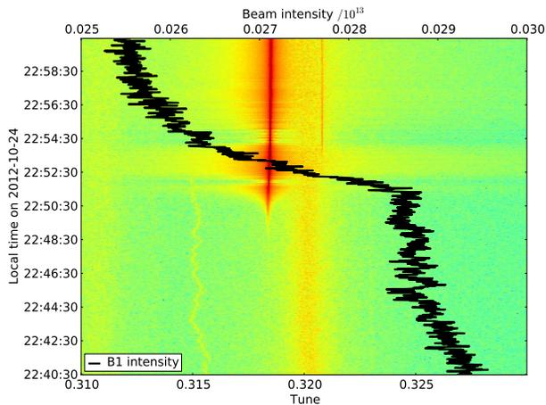
Figure 2: BBQ spectrum versus time for beam 1 in vertical (from an FFT performed on a sliding window) together with beam intensity. The color indicates the amplitude of the spectrum lines.
