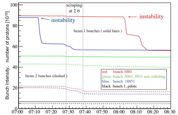
Figure 6: Bunch intensities towards the end of the run, on Oct. 25 from 07:00 to 8:30 hours.
