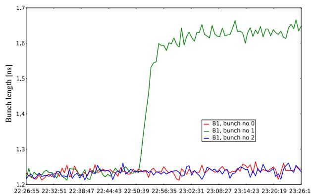
Figure 4: Bunch length evolution for beam 1 over 1 hour around the occurrence of the instability. The color code identifying each bunch is identical to the one used in Figure 1.
