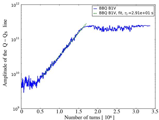
Figure 3: Maximum amplitude of the BBQ spectrum versus time for beam 1 in vertical (from an FFT performed on a sliding window) together with its fit by an exponential.
