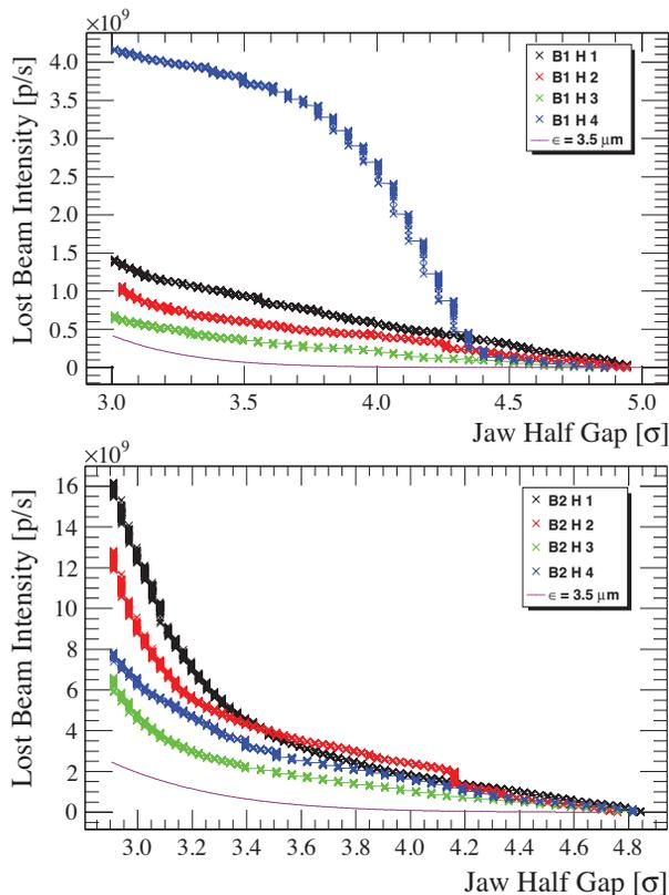
Figure 3: Beam intensity loss as a function of collimator jaw half gap. H 1 to H 4 refers to the successive scrapings.
