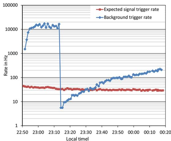
Figure 4: Background trigger rate and signal rate observed in the ATLAS-ALFA Roman Pots.
