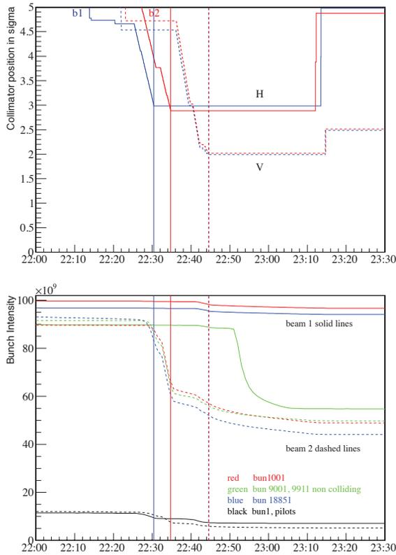
Figure 1: Collimators jaw positions and bunch intensities, 22:00 to 23:30, 1st scraping.
