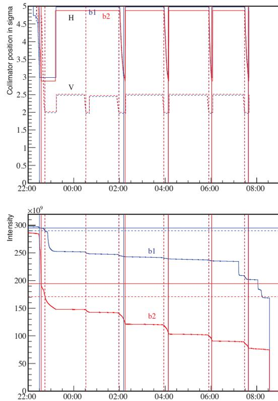
Figure 2: Collimators jaw positions and beam intensities, 22:00 to 09:00.
