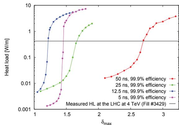
Figure 1: Simulated electron-cloud heat load in the VHE-LHC arc dipoles as a function of the maximum secondary emission yield for different bunch spacings, considering a chamber half aperture of 13 mm, and assuming that 99.9% of the synchrotron radiation photons are absorbed in dedicated photon stops and do not contribute to the primary photoelectrons initiating the EC build up.
