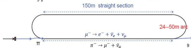
Figure 1: Schematic view of NuSTORM μ storage ring. π<sup>-</sup> → μ<sup>-</sup> scenario is shown. π<sup>+</sup> → μ<sup>+</sup> scenario is obtained by reversing magnet polarities and retuning the injection chicane; with ~same intensity. Arc and straight section lengths will vary when optimized.
