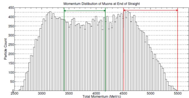
Figure 5:  $\mu$  beam momentum distribution obtained at the end of the stochastic injection straight section from injecting  $5 \pm 0.5$  GeV/c  $\pi$ 's into a NuSTORM straight section of a  $\sim 3.8$  GeV/c  $\mu$  storage ring.
