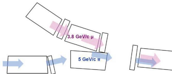
Figure 2: Schematic view of optics for stochastic injection. Pions enter the ring from outside at the dispersion suppressor, joining with circulating lower-energy μ’s. π’s that decay to μ’s within the ring acceptance join the circulating beam.
