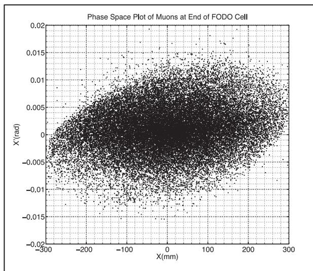
Figure 6: Transverse phase space distribution of muons at end of stochastic injection straight.
