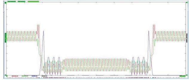
Figure 4:  $\mu$  Lattice functions for a full turn of the storage ring, beginning at the center of the injection straight.
