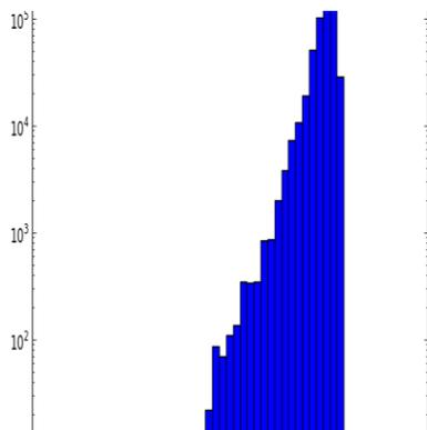
Figure 3: Pulse height distribution of the analog signal from one quadrant.
