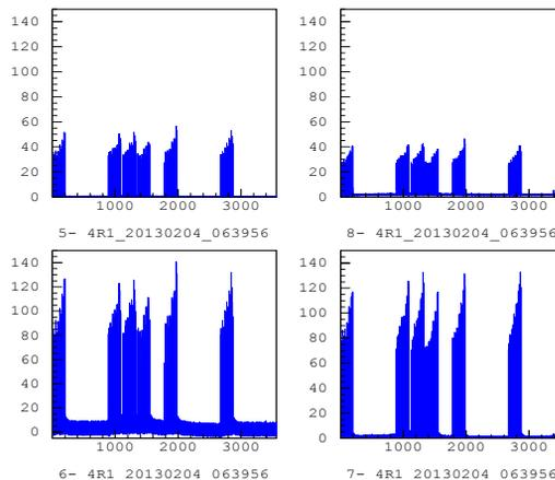
Figure 4: PH-mode in ATLAS with *p-Pb* operation. The plot is taken on the detector at the Right side of the IP which captures the shower from the Lead beams.
