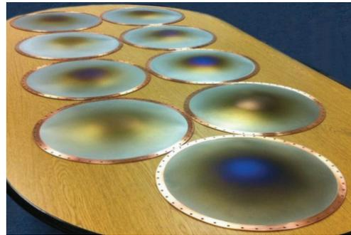
Figure 6: TiN-coated beryllium windows for the RF cavities. The nine windows delivered first are shown.
