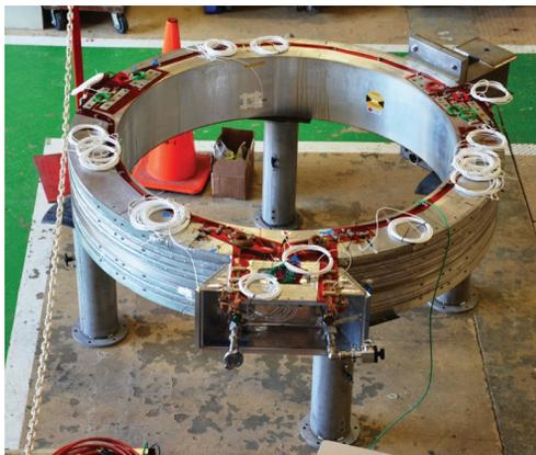
Figure 8: Coupling coil cold mass at Fermilab where it will be tested and trained.
