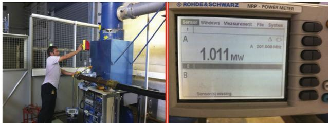
Figure 7: RF amplifier under test at Daresbury.
