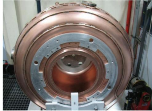
Figure 5: RF cavity after electropolishing.
