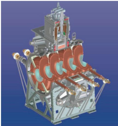
Figure 4: Cutaway of a CAD drawing of an RFCC module. There will be two such modules in Step VI.
