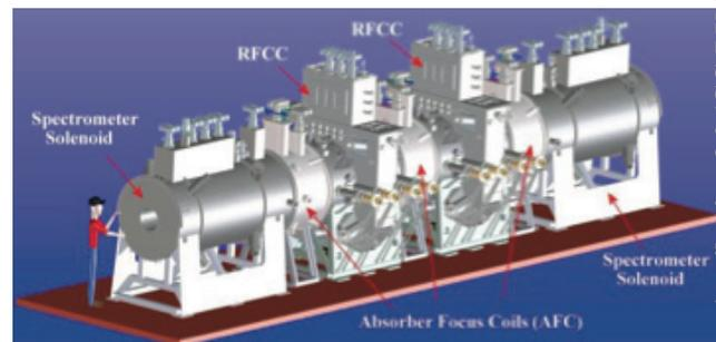
Figure 2: CAD drawing of the fully assembled MICE experiment.
