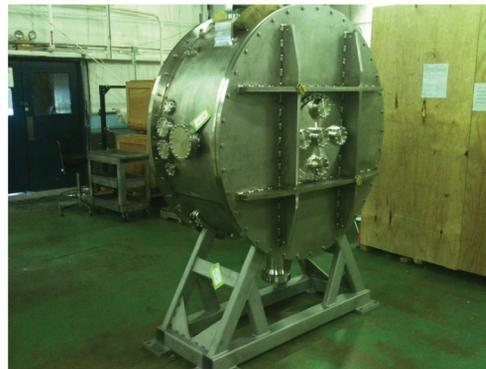
Figure 9: Single-cavity test vacuum vessel at Fermilab.
