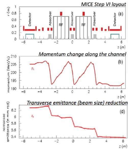
Figure 3: Simulation of 205 MeV/c particles traversing the MICE experiment.
