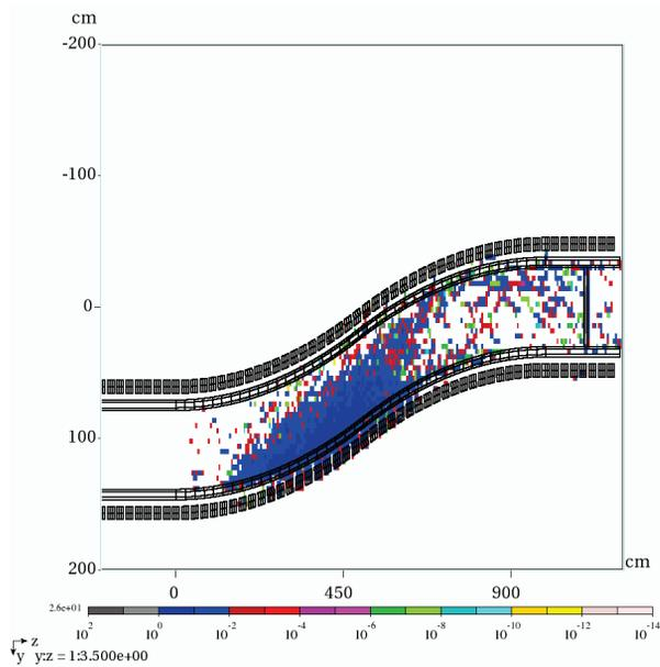
Figure 5: Non-uniform energy deposition in the coils, protons.
