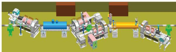
Figure 2: Layout of the two electron lenses in IR10. In 2013 the Blue lens (left) has the EBIS spare solenoid installed instead of the superconducting solenoid designed for the electron lens. In each lens three beams are present, the two proton beams and the electron beam acting on one of the proton beams. The proton beams are vertically separated.
