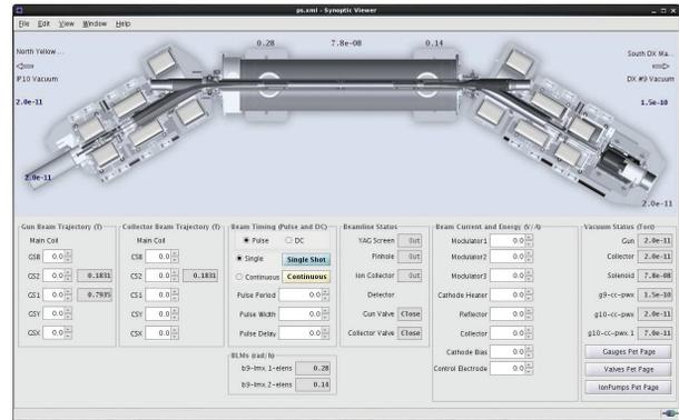
Figure 5: Synoptic display of the electron lens with all high-level data and control points.
