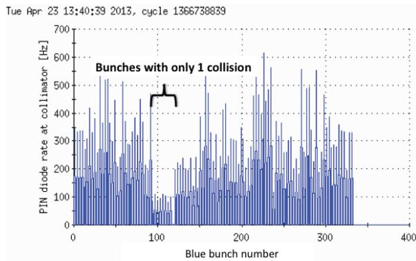
Figure 1: Bunch-by-bunch loss monitor showing lower loss rates for bunches with only 1 collision.
