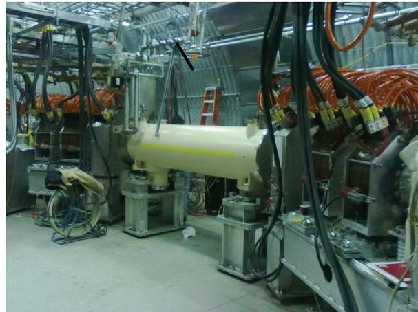
Figure 3: Yellow electron lens as installed in 2013. Visible are the gun side (left), the superconducting main solenoid (center), and the collector side (right).
