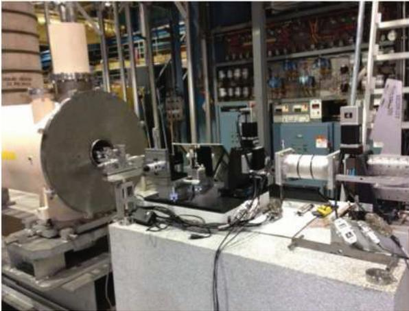
Figure 4: Test setup for the solenoid field straightness measurement in the BNL Superconducting Magnet Division using one of the two superconducting electron lens solenoids.
