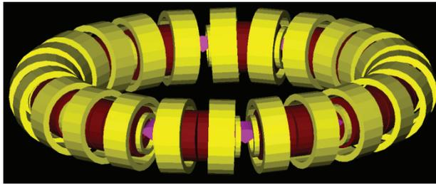
Figure 2: Close view of one of the rings assumed in our computational model. Note that each cell has 4 coils and two of them are rapped around the cavities.
