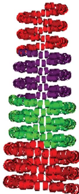
Figure 1: Conceptual design of the first 12 stages of the proposed tapered cooling channel. Different colours label regions of different frequency.
