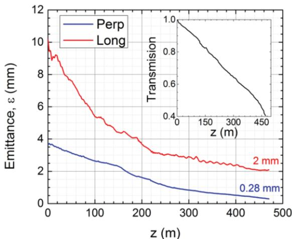
Figure 5: Longitudinal (red), transverse (blue) emittances and transmission as a function of distance along the channel. The final values of the emittances are also shown.
