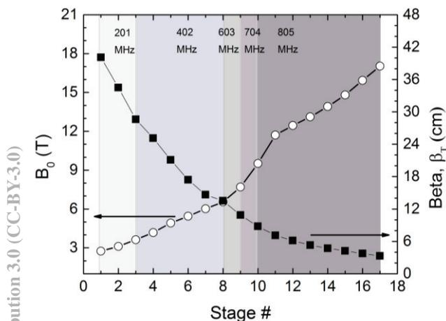
Figure 3: Design value of beta function (right); maximum on-axis field for the solenoid (left). Corresponding rf cavity frequencies are also shown.
