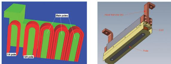
Figure 1: MERMAID model of the wiggler magnet (left); single coil with extended iron core and heat transfer links (right) [5].
