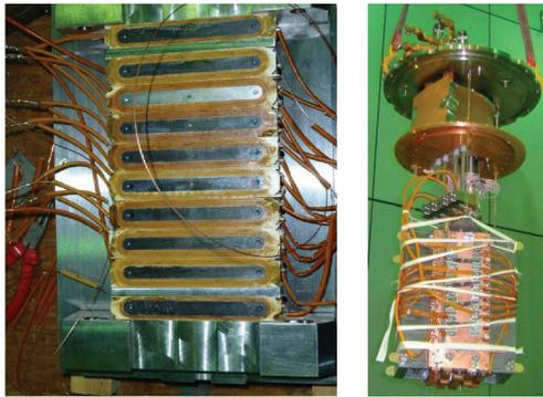
Figure 5: Short model coil assembly (left) and experimental setup for quench and cooling performance test (right).
