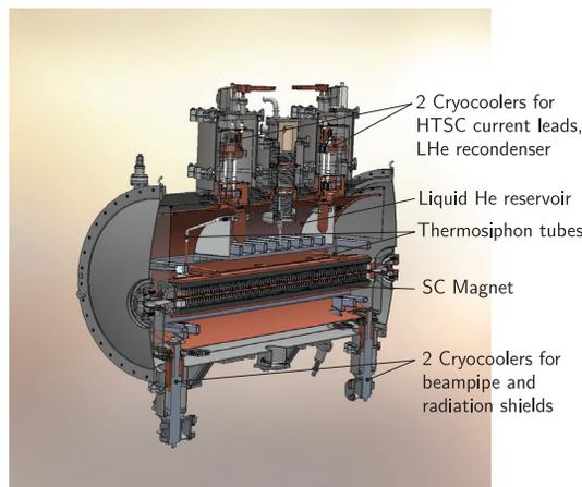
Figure 3: Cross section of the CLIC damping wiggler prototype [5].
