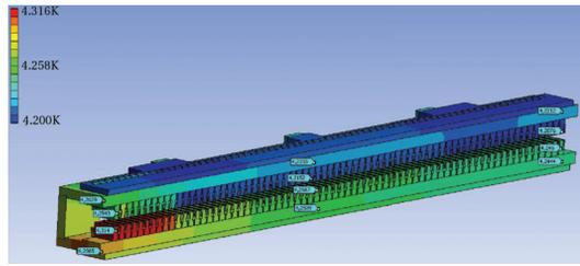
Figure 4: Worst-case estimation of the temperature distribution over the coil arrays of the wiggler assuming that the thermosiphon tubes provide a heat sink at a fixed temperature of 4.2 K and that the first 0.5 m of the beam pipe have a uniform temperature of 70 K and the emissivity of a black body. The maximum temperature at the coil arrays is 4.32 K.
