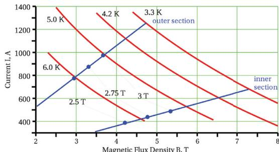
Figure 2: Load lines of the inner and outer coil sections (blue) and critical current as function of  $B$  and  $T$  (red).
