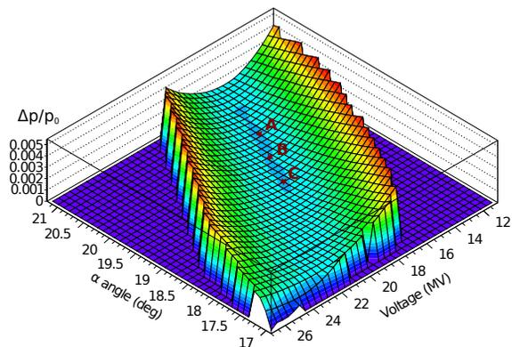
Figure 1: Energy spread of the electron beam at the end of the main linac as function of the parameters of the bunch compressor.
