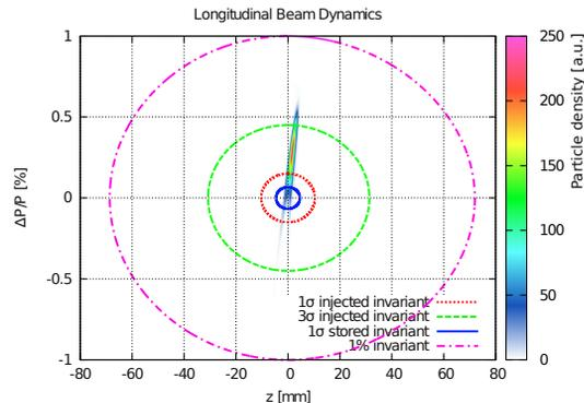
Figure 5: Longitudinal phase space of the injected bunch at septum with a 3 ‰ energy deviation transported in the presented transfer line. The ellipses represent (from inner to outer) the size of the stored bunch, 1σ and 3σ invariants of the bunch injected at reference energy and the 1% acceptance of the ring design.
