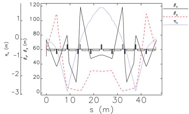
Figure 3:  $\beta$  functions and dispersion for the proposed bending section.
