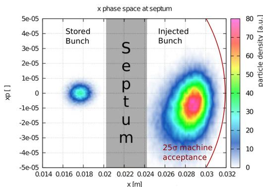
Figure 4: Injected and stored x-phase space of the bunches at septum. The energy error is +3 ‰ with respect to the reference.
