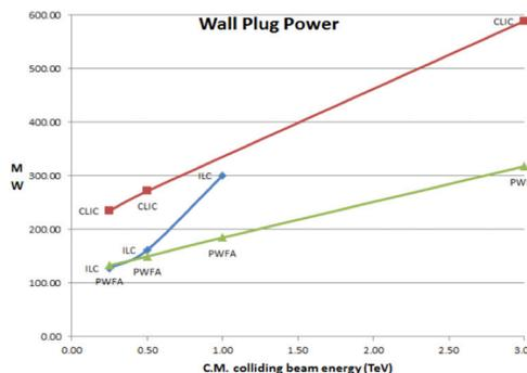
Figure 2: Total wall plug power for a PWFA-LC at various energies, assuming a drive to main bunch efficiency of 50% in the plasma, compared to ILC and CLIC.
