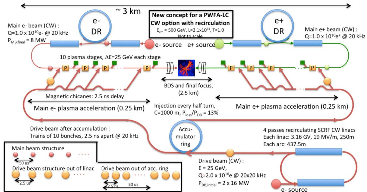
Figure 1: Layout of a 500 GeV PWFA Linear Collider. Each main bunch is accelerated by 25 GeV in each of ten plasma stages. The plasma is driven by  $e^-$  bunches, generated by a SCRF CW recirculating linac, and distributed co-linearly with the main beams.
