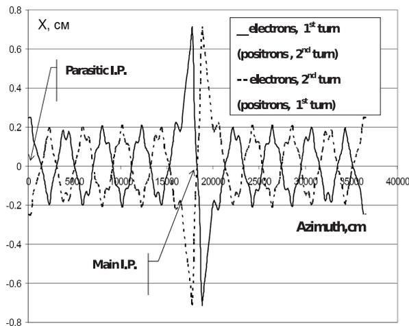
Figure 3: Design radial orbit with the RF separation on.
