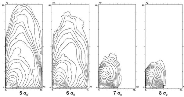
Figure 4: Equilibrium distribution in the plane of normalized betatron amplitudes for VEPP-4M ( $E = 1.85$  GeV,  $I_b = 2.5$  mA), versus the horizontal orbit separation at the parasitic IP. The scales (in units of unperturbed sigmas) are  $15 \times 40$ . The density between successive contour lines drops by a factor of  $e$ .
