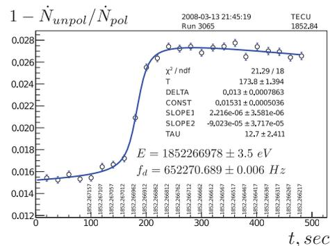
Figure 1: Typical case of the depolarization jump in the relative registration rate of Touschek electrons from the polarized ( $\dot{N}_{pol}$ ) and unpolarized ( $\dot{N}_{unpol}$ ) bunches during scanning of the depolarizer frequency. Scan rate in units of energy is 2.5 eV/s. Depolarization frequency resolution found by the ratio of the experimental data fit error 3.5 eV to the beam energy 1852 MeV is about  $1.9 \cdot 10^{-9}$ .
