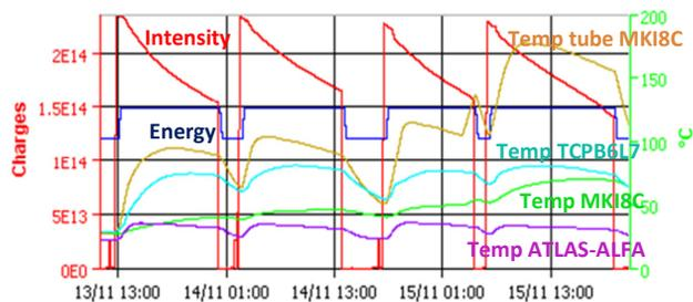
Figure 1: Measured LHC beam intensity (red) and energy (dark blue), along with the measured temperatures of the ceramic tube of the injection kicker MKI-8C (orange), of the skew primary collimator TCP.B6L7.B1 (light blue), of the magnet ferrite of the injection kicker MKI-8C (green) and of the ATLAS-ALFA detector (purple).
