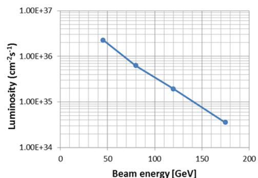
Figure 1: TLEP luminosity per IP multiplied by the number of IPs (four).
