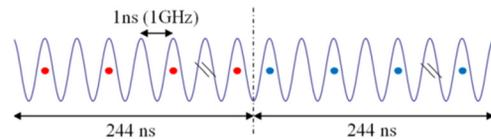
Figure 3: Phase coded Drive Beam.
