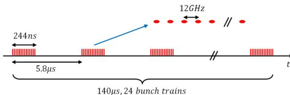
Figure 1: The final time structure of the Drive Beam.
