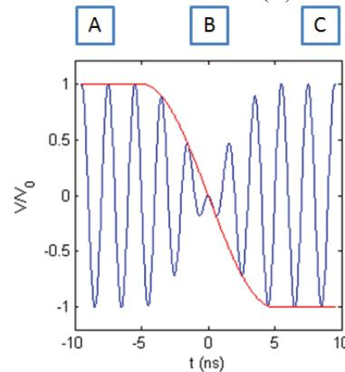
Figure 2: Smooth 180° phase switching model.
