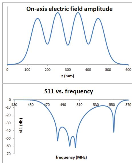
Figure 5: On-axis electric field amplitude and s<sub>11</sub> with a tuned coupler.
