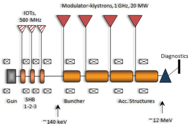
Figure 1: CLIC drive beam front-end layout.
