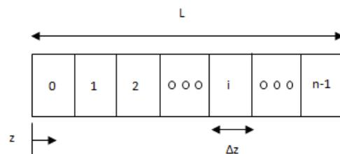
Figure 2: Schematic layout of a forward TW structure.
