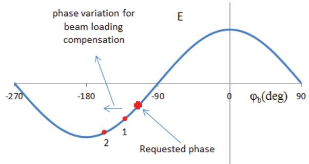
Figure 4: RF source induced field and the bunch related phase progress during crossing the structure.
