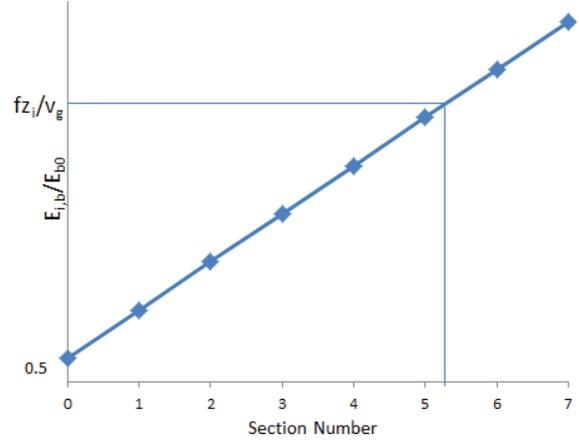
Figure 3: Field evolution inside a TW structure.
