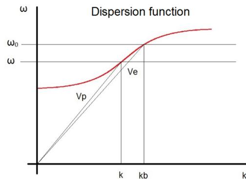
Figure 1: TW structure dispersion function and the meanings of  $\omega$  and  $\omega_0$ .
