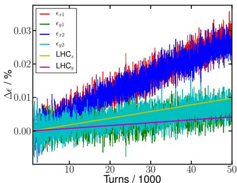
Figure 3: Emittance growth in the HL-LHC with pick-up noise only. The straight lines visualize the measured emittance growth in the reference run in 2012.
