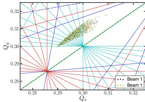
Figure 6: Tune footprint of HL beams. The cyan colored lines represent 10<sup>th</sup> order resonances, red 7<sup>th</sup> order, blue 9<sup>th</sup> order and green 2<sup>nd</sup> order.
