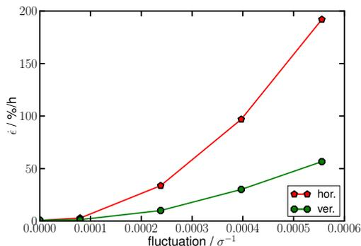
Figure 5: Emittance growth versus noise level on CC phase, average of both beams, expressed as offset at the IP relative to the local beam size.
