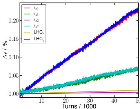
Figure 4: Emittance growth in the HL-LHC with CC noise only. The straight lines visualize the measured emittance growth in the reference run in 2012.
