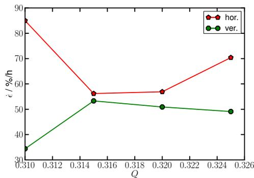
Figure 7: Horizontal and vertical emittance growth versus working point, average of both beams.
