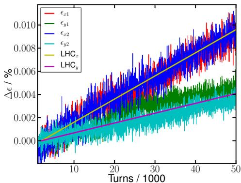
Figure 2: Simulated emittance growth in LHC in 2012. The straight lines visualize the measured emittance growth in the reference run in 2012.
