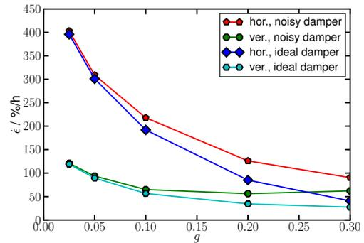
Figure 8: Horizontal and vertical emittance growth versus damper gain, with and without pick-up noise, average of both beams.
