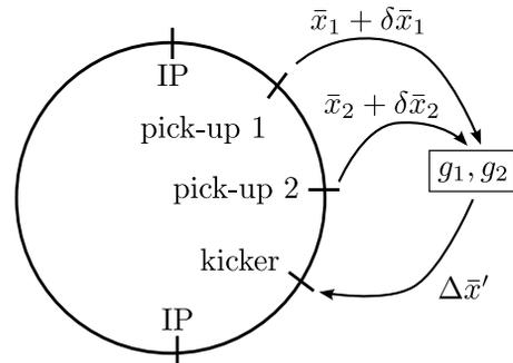
Figure 1: Scheme of the transverse damper.
