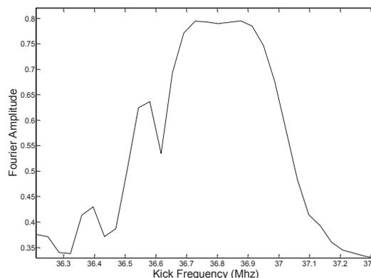
Figure 4: Plot showing the resonant bandwidth for the quadrupole envelope mode in a 23 mA beam.
