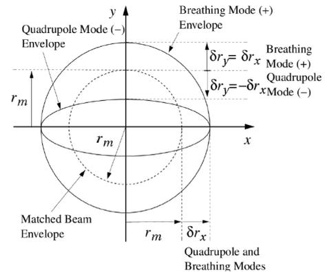
Figure 1: Transverse picture of the envelope modes [4].
