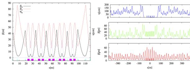
Figure 2: (Left)Optical functions through L0. The light blue rectangles represent quadrupoles and the purple, combined function bending magnets. There is zero dispersion in the RF straights, and zero dispersion in the four straight sections between the pairs of bends. (Right)Twiss parameters for the entire ring. The reconfigured sextant is at  $-60 < s < 60$  m in the right plot.
