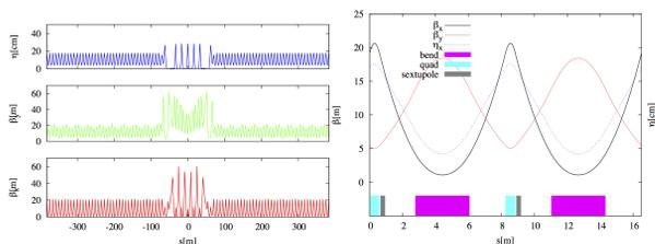
Figure 5: (Left) Penultimate CESR optics. The reconfigured sextant is at the center of the figure. (Right) Arc cell. The bend magnet includes vertically focusing quadrupole and sextupole components. The discrete quadrupole and sextupole are both horizontally focusing.
