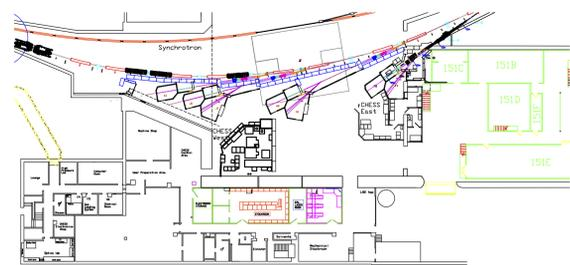
Figure 4: At present CHES x-ray are generated by counterrotating electron and positron beams. In the proposed reconfiguration x-ray lines are all illuminated by radiation from a single beam traveling counterclockwise. A possible layout of undulator beam lines and accompanying experimental stations in the reconfigured machine are shown.
