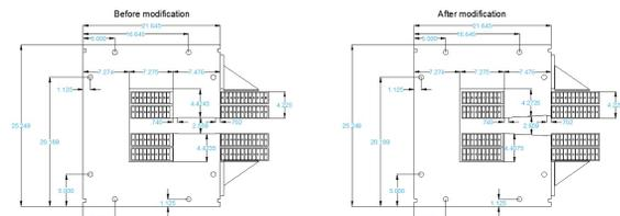
Figure 1: The cross section of the hard bend dipole is shown on the left, and with the pole face modified to provide a vertically focusing gradient on the right.
