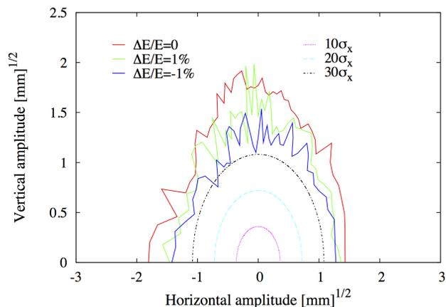
Figure 6: Penultimate CESR dynamic aperture. Lines indicate maximum initial amplitude that survives more than 1000 turns.
