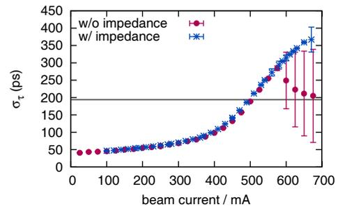
Figure 4: Bunch length evolution with current: The HC potential as well as the geometric impedance lengthen the bunches. The gray line indicates the nominal value of 195 ps at 500 mA
