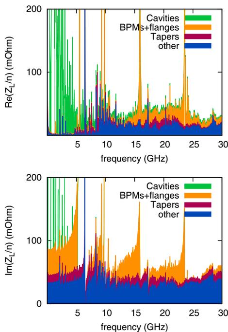
Figure 1: Frequency content of the MAX IV 3 GeV ring longitudinal geometric impedance. The four largest contributors are distinguished. Top: real part. Bottom: imaginary part
