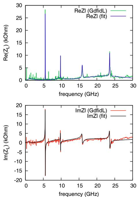
Figure 2: Longitudinal impedance fit to resonators. Top: real part. Bottom: imaginary part.
