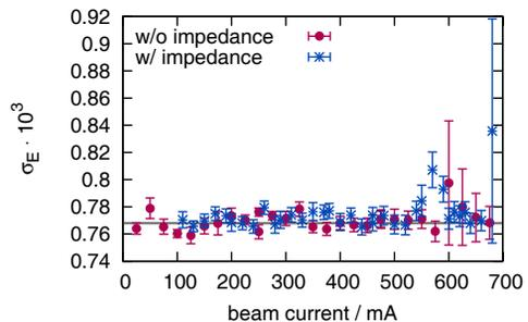
Figure 5: Energy spread evolution with current: Due to the geometric impedance, a clear increase occurs at 550 mA, which is above the planned operating current of 500 mA. The gray line indicates the natural energy spread.
