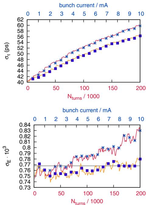
Figure 3: Top: Bunch length evolution with current. Bottom: Energy spread evolution with current. Red: all resonators included. Orange: resonator number 6 excluded. Markers indicate a current increase by 0.5mA after tracking for 10000 turns. The gray line indicates the natural energy spread of  $7.69 \cdot 10^{-4}$ .
