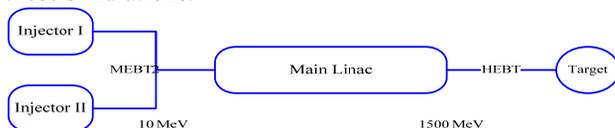
Figure 1: Layout of the C-ADS linac.
