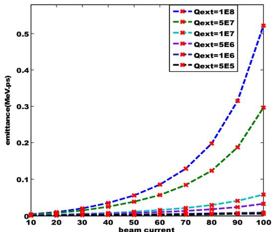
Figure 5: Diffusion against different bunch current for different external damping.
