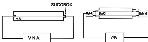
Figure 6: Schematics of longitudinal (left) and vertical (right) impedance measurement with SUCOBOX.
