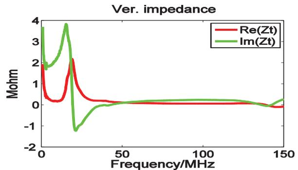
Figure 4: Vertical  $Z_T$  of the RCS fast extraction kicker.
