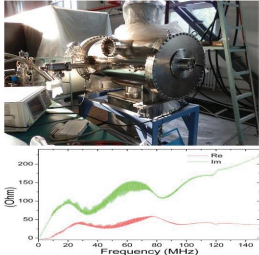
Figure 3: Longitudinal measurement platform (top) and measurement result (bottom) for CSNS/RCS extraction kicker prototype.
