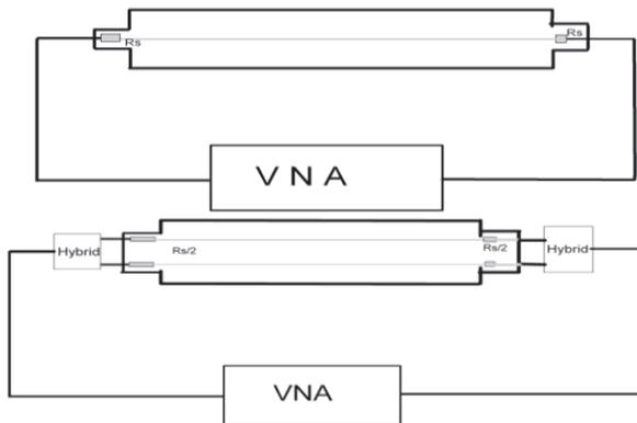
Figure 2: Schematics of longitudinal (top) and transverse (bottom) impedance measurement.
