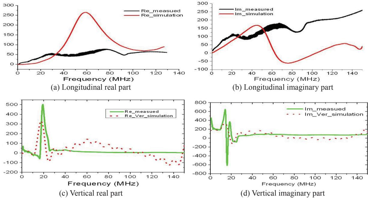
Figure 5: Longitudinal and vertical impedance comparison between measurement and simulation.
