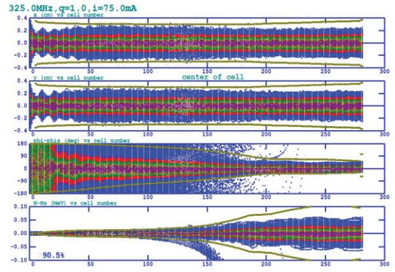
Figure 5: Beam dynamics in the RFQ for the input current of 75 mA, 5000 particles. From top to bottom are: x, y, phi, and energy coordinates versus cell number. The percentage transmission is 90.5%.
