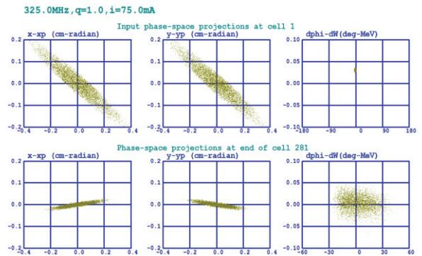
Figure 6: PARMTEQM simulation showing phase-space plots of the input beam and the beam at cell 281.
