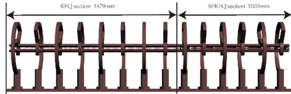
Figure 1: Inter structures of CRS cavity.
