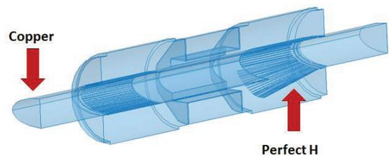
Figure 8: HFSS eigenmode simulation setup.
