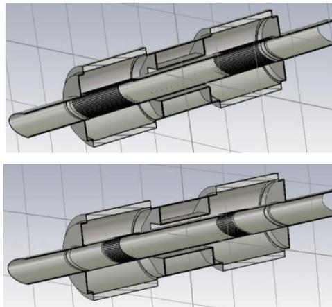
Figure 2: Longitudinal sections of the VMTSA module equipped with the longer RF fingers (top) and shorter RF fingers (bottom). Conforming case.
