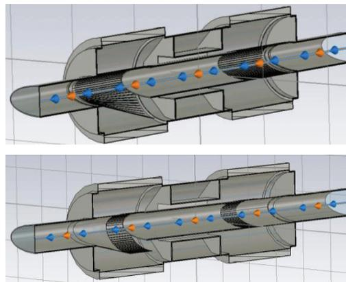
Figure 3: Longitudinal sections of the VMTSA module equipped with the longer RF fingers (top) and shorter RF fingers (bottom). Loss of contact.
