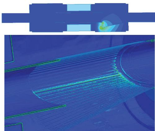
Figure 9: Electric field distribution in VMTSA (top) and surface loss density (bottom, log scale) on the longer fingers for the eigenmode at 279 MHz and 40mm gap.
