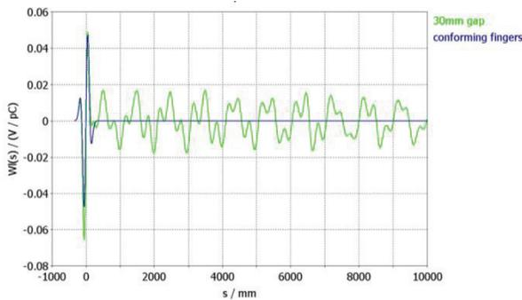
Figure 5: Longitudinal wake potential for conforming fingers (blue) and 30mm deformation (green).
