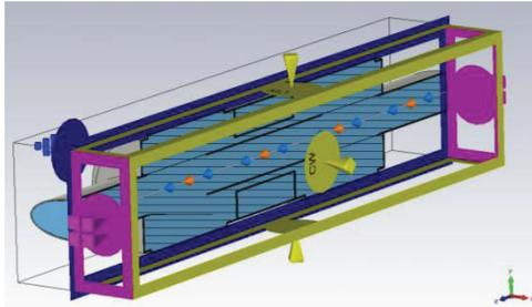
Figure 4: Time domain simulation setup of VMTSA equipped with the longer deformed RF fingers.
