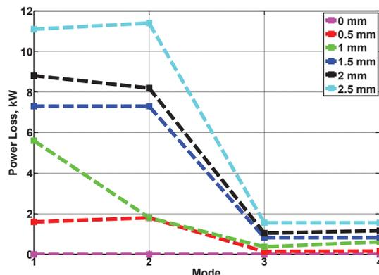
Figure 10: Power loss dependence on the gap size for the the VMTSA module equipped with the short RF fingers.
