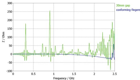
Figure 6: Longitudinal wake impedance for conforming fingers (blue) and 30mm deformation (green).
