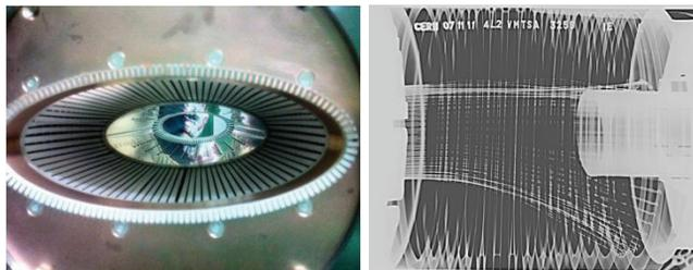
Figure 1: Conforming RF fingers as installed in the VMTSA module (view from beam-pipe at left) and X-ray image of the deformed fingers (right).
