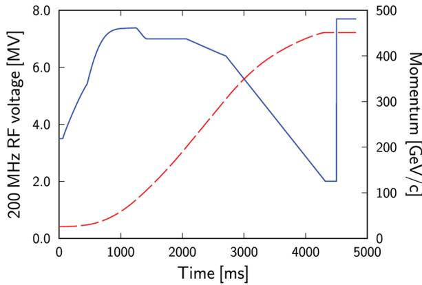
Figure 1: Beam momentum (dashed line) and 200 MHz RF voltage programme (solid line) used during Q20 measurements. Flat top and bunch rotation (with 1 ms voltage rise) start at cycle times 4320 ms and 4500 ms, respectively.
