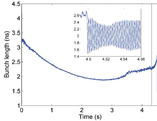
Figure 2: Typical bunch length ( $4\sigma$  Gaussian fit) evolution during the cycle in the Q20 optics, at  $3.73 \times 10^{11}$  p flat top intensity. The vertical line marks the beginning of the flat top. The inset shows the arrival to flat top and subsequent rotation in more detail. The bunch should be extracted after 1/4 of the synchrotron period.
