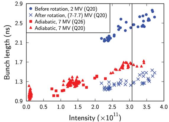
Figure 3: Flat top bunch length ( $4\sigma$  Gaussian fit) before and after rotation as a function of intensity. The vertical line marks roughly the threshold of stability in Q20.
