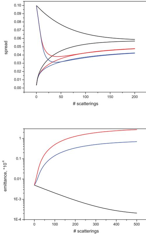
Figure 1: Spreads (top) and the emittance (bottom) vs number of scatterings for nondispersive (black), uncoupled (red) and coupled (blue) dispersive CP.
