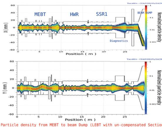
Particle density from MEBT to beam Dump (LEBT with un-compensated Section)
