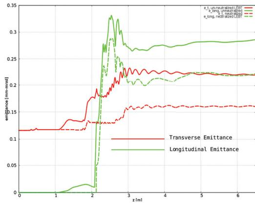
Figure 4: Emittance evolution through the RFQ. Solid: LEBT with un-neutralized section. Dashed: Fully neutralized LEBT.
