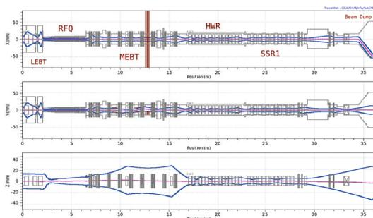
Figure 1: PXIE end-to-end  $3\sigma$  beam envelopes. Top:  $(x, x')$ , Middle:  $(y, y')$ , Bottom:  $(z, z')$ . The MEBT is in shown operating in transmission mode. The beam sweep magnet is shown steering horizontally over the dump area.
