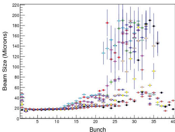
Figure 2: The vertical beam size of bunches for trains of varying lengths plotted vs. their 4 ns bucket number. The colors of the points correspond to trains of different number of bunches: 30(red), 30(teal), 32(green), 32(orange), 34(blue), 34(magenta), 36(violet), 36(tan), 38(gray), 38(yellow), 40(black) and 40(brown).
