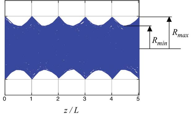
Figure 2: Matched beam in periodic focusing structure.
