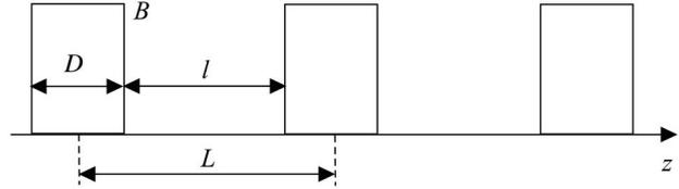
Figure 1: Periodic structure of focusing solenoids.
