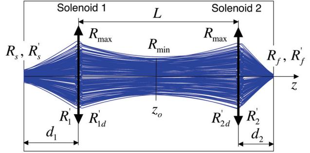
Figure 3: LEBT with two focusing solenoids.
