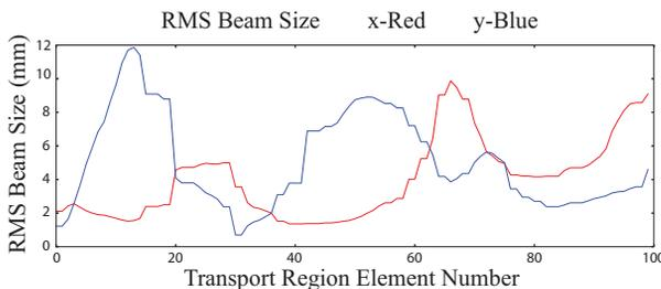
Figure 5: RMS beam size at the end of the iterative tuning scheme.
