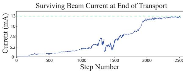
Figure 3: The surviving current at the end of the beam transport over 2500 iteration steps is shown for an initial beam current of 13mA.
