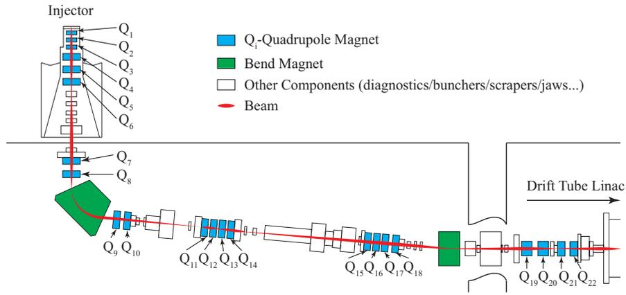
Figure 2: Simplified schematic of the LANSCE  $H^+$  injector and transport region.
