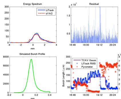
Figure 3: Comparison of LiTrackES with TCAV and Pyrometer over a four hour period. Note that the pyrometer varies inversely with bunch length.
